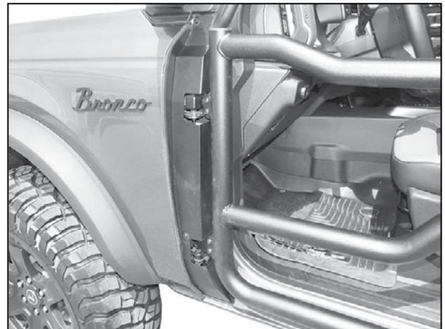
(Fig 9) Adjust fit of Cover and fully tighten all hardware
